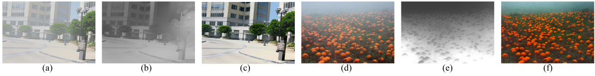
Figure 1: Haze removal of single image using our method: (a) Input hazy image (simulated haze). (b) Estimated transmission map of (a). (c) Our haze removal result of (a). (d) Input hazy image (real haze). (e) Estimated transmission map of (d). (f) Our haze removal result of (d).
