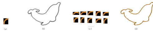
Figure 4: Generation of strokes. (a)Sample stroke. (b)Empty stroke divided by 200 small quadrangles. (c)Rotating the sample stroke. (d)Result of synthesis.
