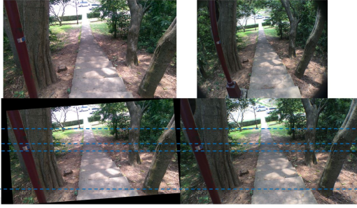
Figure 2: Example of rectification on real stereo images: the input stereo images (first row) and rectified images with auxiliary lines (second row).
