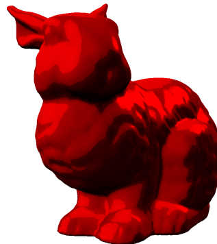
Figure 1: A toon shaded Stanford bunny of 70K triangles rendered as a resolution-independent planar map of visible triangle portions (depth complexity is no greater than one) in about 15 ms (67 Hz) by the SVGPU vector renderer, representing more than a four-fold improvement over previous GPU vector renderers.
