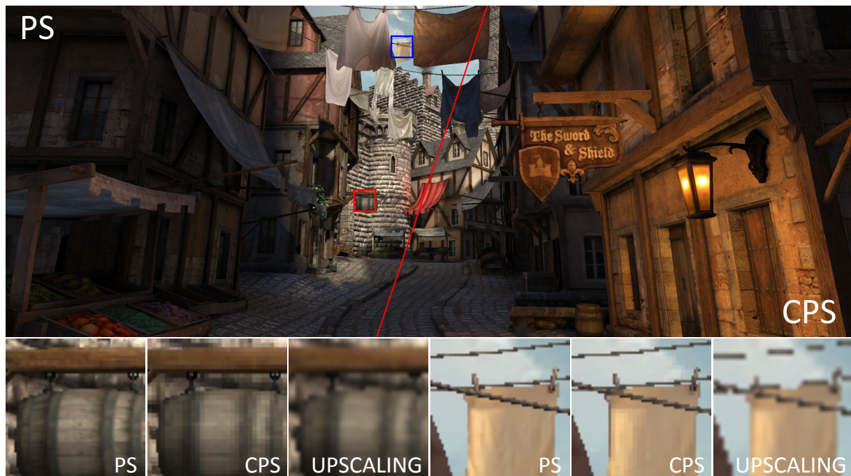
Figure 1: The CITADEL 1 scene, rendered at 2560 \times 1440 with pixel-rate shading (PS) on the left and coarse pixel shading (CPS) on the right, using a coarse pixel size of 2 \times 2 . CPS almost halves the number of shader invocations, yet shows few perceivable differences on a high pixel density display, with a structural similarity index (SSIM) of 90.6%. In contrast, an image rendered at 1280 \times 720 and upscaled exhibits blurring at silhouette edges, and lower overall quality, with an SSIM of 86.9%.
