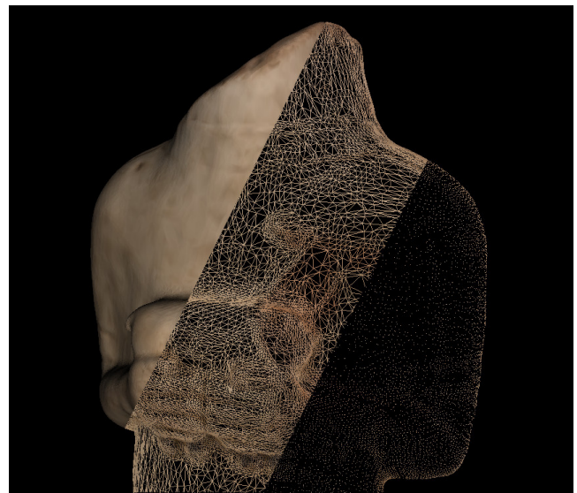
Figure 4: The three available visualization modalities for 3D fragments: solid (left), wireframe (center) and points (right); these modalities are available for all the 3D-related views.
