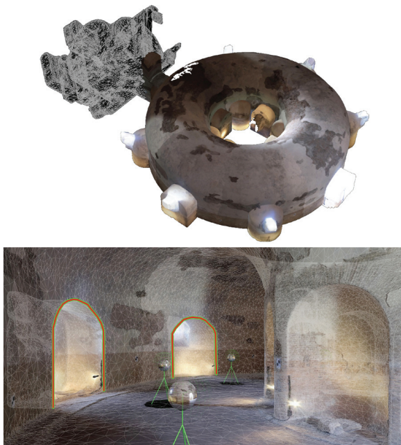
Figure 11: Texturing in 3D Studio Max (top) textured model (bottom) The correct alignment is evident near the niches: green and red lines correspond.
