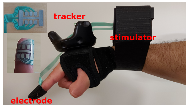
Figure 2: Experimental apparatus. The electrical stimulator is attached to the forearm and the electrode is placed in contact with the finger pad. The two insets represent detailed views of the electrode. The user's hand is tracked by a HTC Vive Tracker.
