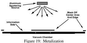
Here, the transparent CDs are coated with a thin aluminum layer in a process similar to an electrostatic discharge; this layer makes the discs reflective. The manufacturer checks the first discs to be metalized, both visually and electronically, for defects in the stamper qualification process. Discs are verified, byte-for-byte, against the original customer-supplied source material,
