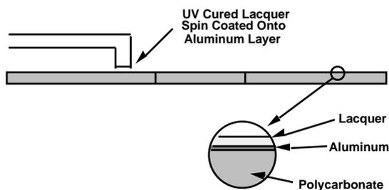
Figure 20: Protective coating with cross-section of disc layers
