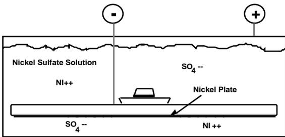
Figure 15: Electroplating
