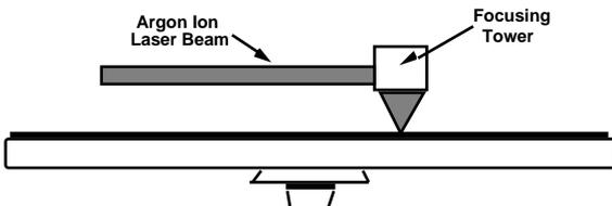
Figure 11: Laser writing on the blank
