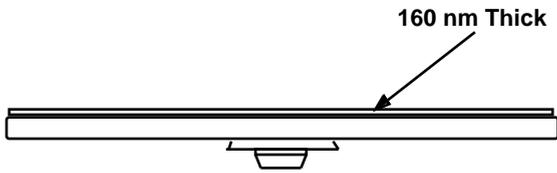
Figure 10: Photoresist layer
