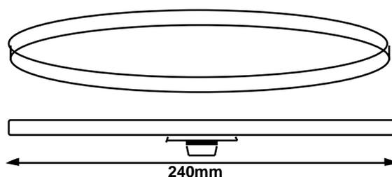
Figure 9: Glass substrate on mounting hub
