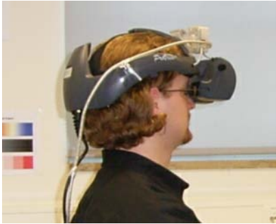
Figure 6: Head-mounted display (HMD), shown here in a configuration with a camera for use in augmented reality.
