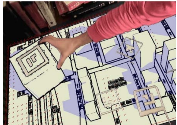
Figure 13: Selective stylization for augmented reality in a tangible user interface. This image shows an augmented urban planning application. The building model held by the user is a real object, while the city plan shown beneath the user's arm is virtual.
