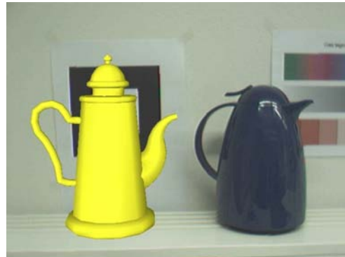
Figure 8: Augmented reality scene showing a real tea pot (seen at right) and a virtual tea pot model (seen at left). This image shows a conventional AR representation.
