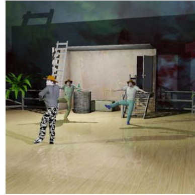
Figure 1: This dynamic scene with 63k static and 171k animated triangles can be ray traced with 7.2fps at 1024^2 pixels on a four core 3GHz Intel Core 2 Duo including shadows from two point lights [SSK07].
