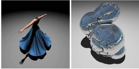
Figure 6: Two screenshots from Lauterbach et al.'s BVH based ray tracing system. Left: One frame from a 40K tri-angle dress simulation animation, running at 13 frames per second ( 512 \times 512 pixels, one point light) on a dual 2.8GHz Pentium IV PC. Right: a fracturing bunny including shadows and reflections, running at an average of 6 frames per second on same hardware.
