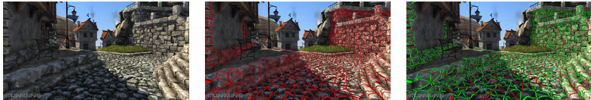
Figure 1: Left: A frame from Heaven 2.0 running in our simulator. Center: Redundant shading work (red) occurs along shared patch edges. Right: Savings from an eight-entry edge cache (green).
