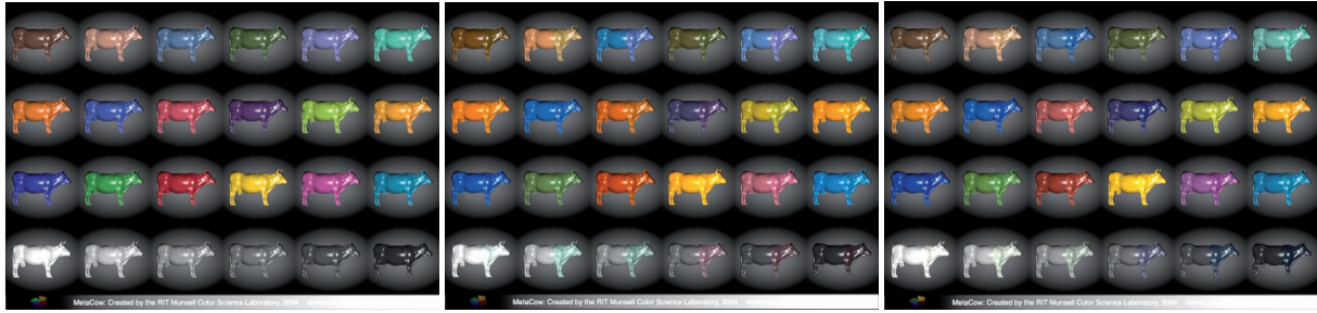
Figure 1: A replication of the Metacow image rendered with our spectral PRT method. Left: Illuminant D65, center: Illuminant A, right: Illuminant F2. RGB rendering would not resolve the metamers under illuminants A and F2.
