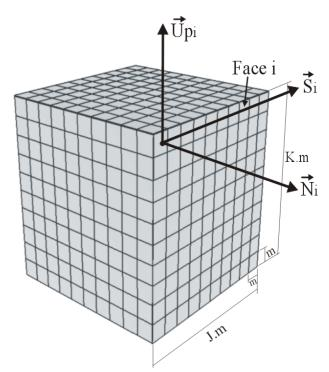
**Figure 2** – Each face *i* has a local coordinate system, formed by the vectors  $(S_i, Up_i, N_i)$ . Each face must have its own base transformation matrix  $T_i$ , which converts a local coordinate to the global coordinate system.
