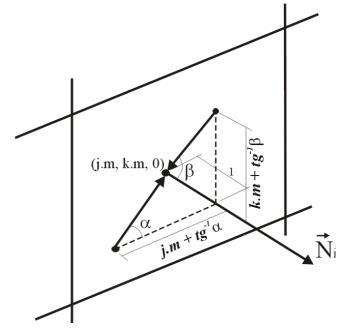
**Figure 3** – In order to obtain the angles where the accumulated density is evaluated it is necessary to apply regular increments to  $\alpha$  and  $\beta$ .
