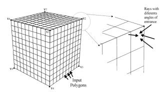
**Figure 1** – The volume is represented by a geometric object (a box in this figure), which is divided in input polygons. Each of those polygons have a table with different input angles. It stores the density accumulation along the ray path relative to each input angle.
