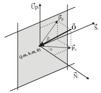
**Figure 4** – Evaluation of angles  $\alpha$  and  $\beta$  which are formed between vector O and the local coordinate system of the face the current polygon belongs to.
