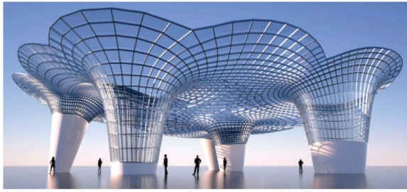
Figure 28: Constrained meshes, i.e., the shape space of meshes with a set of prescribed constraints involving the free vertices, preserve non-local part relations while allowing the users to directly navigate in the implicitly defined constrained shape space [YYPM11].
