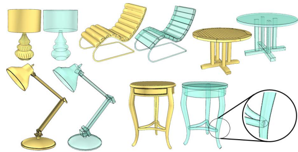
Figure 15: Controllers (shown in cyan), either a cuboid or a generalized cylinder [ZFCO*11], serve as high-level deformation handles for structure-aware deformation of man-made shapes [XZZ*11]. The numbers indicate the number of controllers needed, showing that a small number of controllers usually suffice for the modeling tasks.
