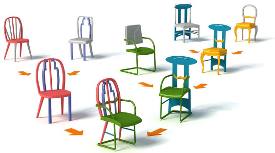
Figure 22: Evolution paths leading to the generation of a chair (bottom) with a new structure [XZCOC12]. Note that new topologies can be generated by the crossover operator. The ancestors of the final chair belong to sets of shapes that are evolved together; i.e., a set evolution.
