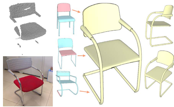
Figure 27: Structure-aware 3D model reconstruction from Kinect data. The reconstruction is based on retrieving and then assembling parts taken from multiple example shapes in a small shape repository, while preserving the built-in structures of the examples [SFCH12].
