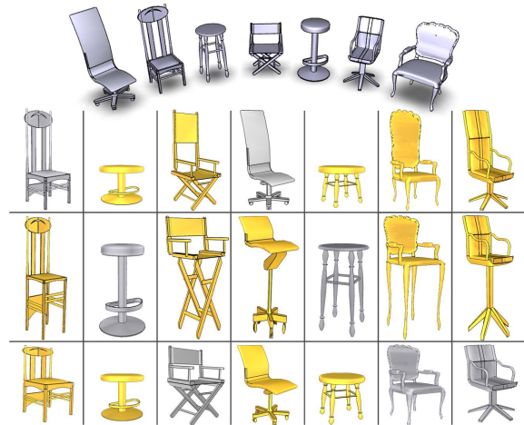
Figure 10: Style-content separation [XLZ*10] by anisotropic part scales facilitates part correspondence among a diverse set of chairs (top). The separation is shown by the table with rows representing identified styles. The correspondences allow automatic synthesis of novel shapes (shaded in gold) from the example set via style transfer.
