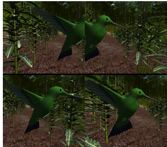
Figure 3: The adjustment system in effect. Top: An unadjusted setup, matching the physical HMD. Bottom: Both eyes adjusted. The direction from each eye towards the hummingbird would appear parallel.
