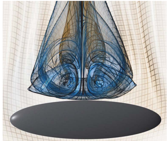
Figure 6: Streamsurface of the ellipsoid dataset rendered with normal-variation transparency, grid-like texture and silhouette enhancement (image courtesy of Hummel et al. [HGH*10] ©2010 IEEE).
