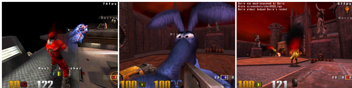
Figure 2: Student hand-ins of 2005. Left to right: Motion blur (using render-to-texture), Fur shader (using a pixel shader), Burning player models (particle effect).
