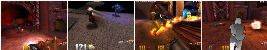
Figure 1: Various 3D effects implemented by students in 2006. Left to right: Environment mapping (level reflecting on a sphere), Motion blur (using Render-to-Texture), Particle effect, Toon shader (fragment shader).
