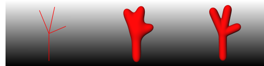
Figure 5: Transition at branching, left: skeleton, middle: convolved with original filter, right: convolved with modified filter
