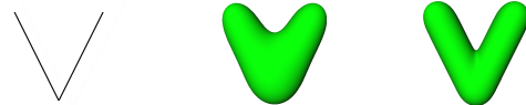
Figure 2: Blending strength, left: skeleton, middle: high blending strength, right: reduced blending strength
