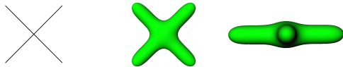
Figure 3: Bulging problem, left: skeleton, middle: convolution surface, right: Bulge at the branching in horizontal view
