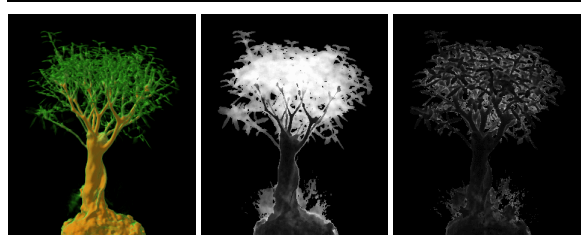
Figure 6: Number of sampling steps for different transfer functions: On the left the original image is depicted and at the center the corresponding number of sampling steps is shown (White corresponds to 512 samples). On the right a more opaque transfer function was chosen to illustrate the impact of early ray termination.
