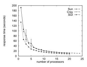
Fig. 3. Response time for SGI Challenge, Sun SparcCenter 2000, and Cray CS6400 with a 500 base sequence using parallel BLASTX SMP algorithm.
