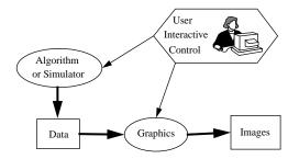
**Fig. 1.** Existing steering model. The simulation generates data that is given to a visualizer to generate the images on the screen. The user can interact with parameters of the algorithm and manipulate the objects on the screen.
