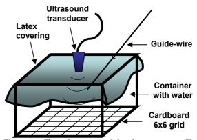
**Figure 1:** This schematic is of the phantom setup. The latex-covered container filled with water simulated the body. The grid acted as target points within the body, and the guide-wire represented the catheter ablation probe.
