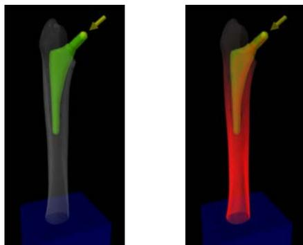
**Figure 1:** Screenshots of the simulation environment: Left: Semi-transparent rendering of the femur and the implant (green color) as well as the volume rendering of the femur's interior structures support the positioning of the implant. Right: The load on the femur is indicated by the yellow arrow and sphere, and the resulting stresses in the volume are visualized with red color.
