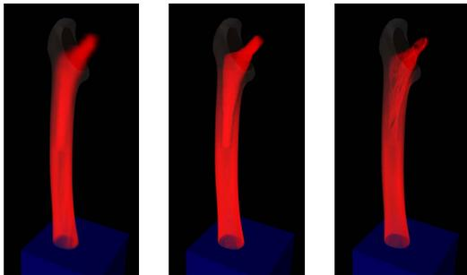
**Figure 3:** Stress visualization using per-element stress (left) and sub-element stress (middle) for a FE model resolution of  $8^3$  CT voxels/hexahedron. For comparison, we also show the stress computed on the initial CT resolution (right).
