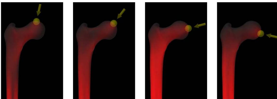
**Figure 7:** Visualization of the (per-element) stress for various load directions using a FE model resolution of  $4^3$  CT voxels/hexahedron.
