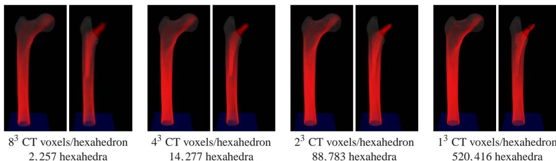
**Figure 4:** Visualization of the (per-element) stress distribution inside the bone at different FE model resolutions, without and with the implant. Note that the principal stress distribution can already be deduced from the coarsest resolution, while at the highest resolution, the trabecular structures of the femur (right) are visible.
