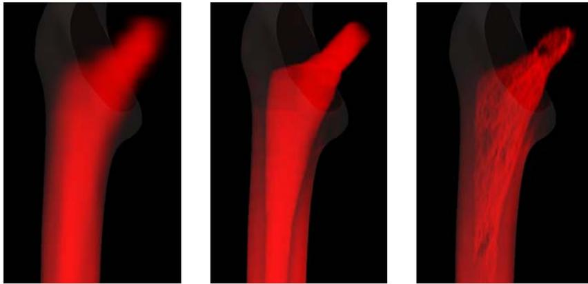
**Figure 5:** Stress visualization using per-element stress (left) and sub-element stress (middle) for a FE model resolution of  $8^3$  CT voxels/hexahedron. For comparison, we also show the stress computed on the initial CT resolution (right).
