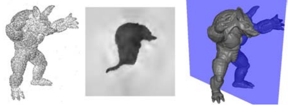
Figure 2: Points from scans of the “Armadillo Man” model (left), our Poisson surface reconstruction (right), and a visualization of the indicator function (middle) along a plane through the 3D volume.
