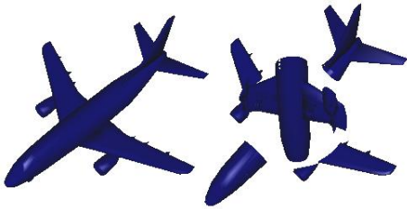
Figure 5: The model on the right is obtained by applying a rotation to the interior part of the model on the left. While the models are not rotations of each other, their Spherical Harmonic Representations are the same.
