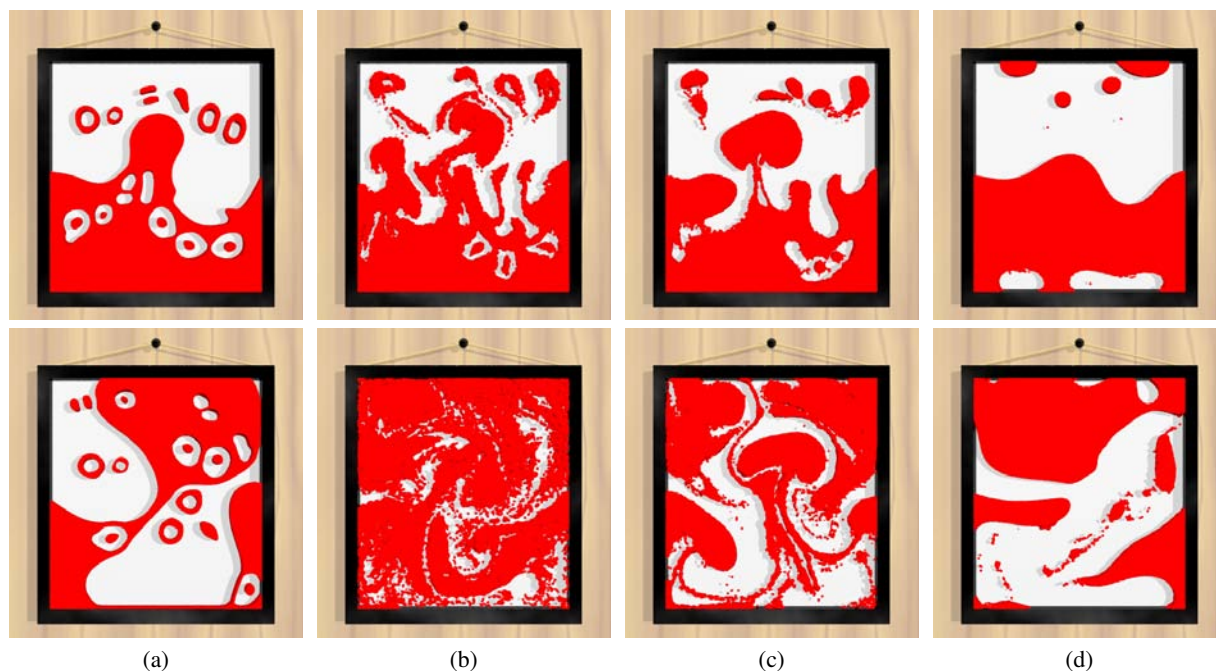
Figure 6: Two fluids with a density ratio of 10 at two different points in time. While standard SPH produces unnatural interface tension (a), our method prevents any spurious tension between the fluids (b). As a result, interface tension forces can be added with full control, (c) and (d) show a tension strength of \sigma = 5 and \sigma = 35 , respectively.
