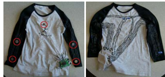
Figure 1: Left. The outside of the shirt shows the location of the accelerometers (circled in red). Right. The traces on the inside of the shirt are laid out to minimize crossings.
