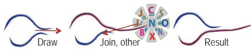
Figure 3: The user drew a stroke that the system assigned to the wrong curve. The user over-rides that choice by tapping on the end of the stroke, which brings up the stroke menu. The user can pen-down on the “join” option and draw to the desired curve. Menu options, from top clock-wise: Combine two curves, Smooth the join, Oversketch, New closed curve, Delete, Back-and-forth scratch, Join, Join and close. Center option is for New curve.
