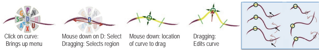
Figure 4: Dragging a part of a curve. The user selects the curve (one click) then selects the drag option and the region of the drag on the curve (pen-down in option, drag over curve region). They can then grab and drag the curve in the direction of the view plane, or along the view plane normal (clicking on top or bottom of drag arrow). Right: Translating, scaling, and rotating the curve are also invoked from the menu, with the specific operation determined by where the cursor is with respect to the drag icon (circle) and curve (above or below).
