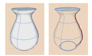
**Figure 4:** Left: a subdivided surface of revolution. Thin blue lines show the structure of the control mesh. Right: a "widget" lets the user overksetch the thick blue cross-section curves or the red profile curve to modify the shape.
