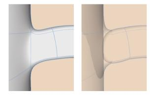
Figure 1: Left: two surfaces blended together (normal view). Right: interior view showing original surfaces, plus the layer of "skin" that joins them.
