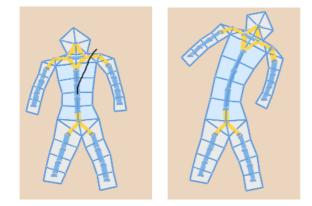
Figure 3: Left: a paper-doll consisting of 10 panels; thick blue lines/dots denote the spines of panels, and the yellow lines connects them together; the user is oversketching a spine. Right: the result of the oversketch.
