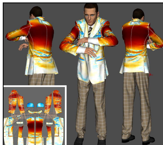
Figure 7: Virtual prototyping applications require an accurate representation of cloth material behavior for evaluating precisely the stretch forces (color scale) on the garment in particular postures of the character.
