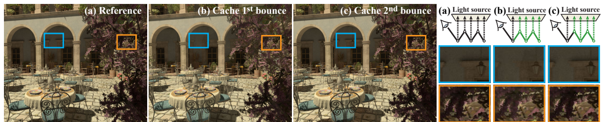
Figure 1: Our visibility caching significantly speeds up tracing of secondary rays, here from 0.15 MRays/s (reference) to 0.70 MRays/s (with the visibility cache). The images were rendered using path tracing where some of the rays (highlighted by green in the illustrations; solid and dashed lines represent path segments and shadow rays, resp.) were traced using our visibility cache with 2000 shadow maps achieving 4.7\times higher throughput of secondary rays per second.
