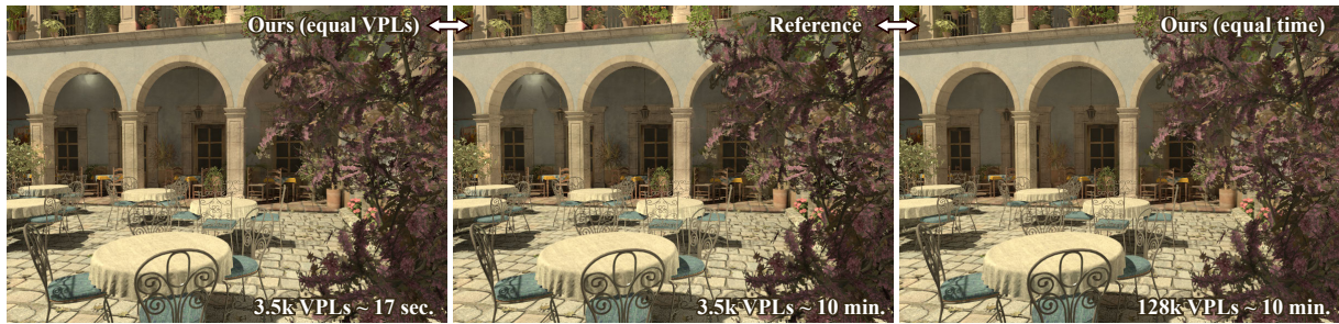
Figure 6: GPU-based VPL rendering of indirect illumination in the San Miguel scene (24M triangles): our shadow map-based caching of visibility (left and right) renders 36× faster than the traditional approach (middle), where shadow maps are created for each VPL. The traditional VPL rendering shows artifacts (e.g. the bright splotch in the arcade) even after 10 minutes.
