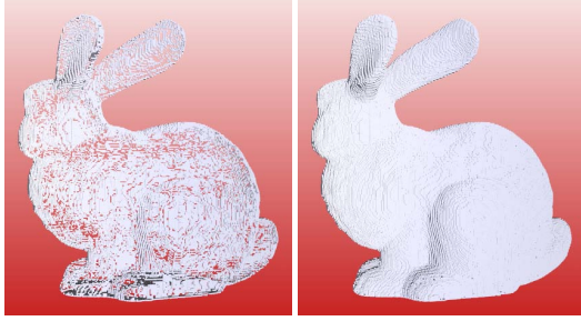
Figure 5: Comparison of the voxelization using the pixel shader clipping method at 256^3 volume resolution with 3 and 9 geometry shader vertices output. The number of voxels produced are 52382 and 89696 (complete voxelization) respectively.
