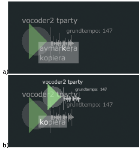
Figure 6: First and second key press while the cursor hover over a sound component. (a) Feedback of the command that in this context match the typed key is displayed. (b) The first command of the list is due to be invoked, indicated by the stronger contrast. Note that a pre-visualisation of the copy command is also shown.
