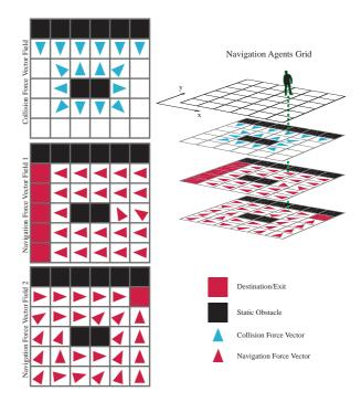
**Figure 2:** An example of a simplistic 6x6 environment with 2 exits and obstacles. Navigation agents are arranged in a grid as shown (top right) and position of the agent relates to a particular cell of the force vector fields.
