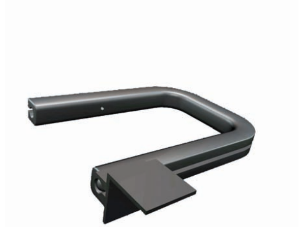
Figure 5: The proposed base rail for manipulator's motion around the wheelchair
