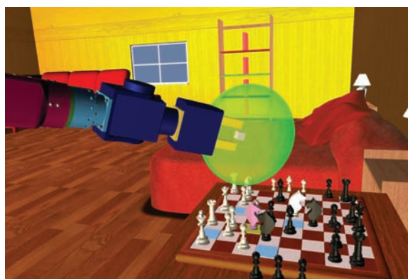
Figure 8: Execution of the task at a chessboard: the manipulability ellipsoid is displayed on the screen
