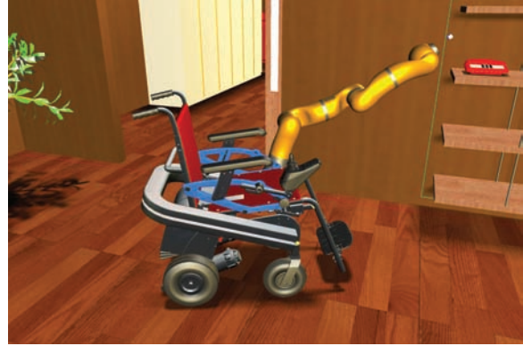
Figure 2: The virtual environment with a wheelchair-mounted manipulator on a sliding rail
