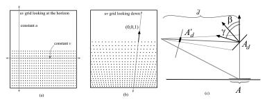
**Fig. 6.** (a) If we look straight at the horizon, the projected grid is uniform. (b) If we look down, there is distortion. The elevation occurs along the constant u line in image space, facilitating occlusion culling. (c) Undersampling factor F geometry. (d) Occlusion culling for terrains.
