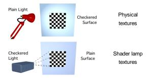
Figure 2: Concept of *shader lamps*.
