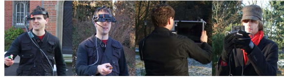
Figure 1: The compared devices: Monocular Head-Mounted Display, Binocular Head-Mounted Display, Tablet PC and UMPC (from left to right).
