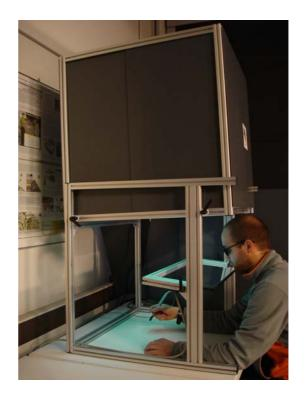
Figure 1: Current prototype of the PDRIVE, the Projectorbased, Desktop, Reach-In Virtual Environment.
