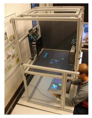
Figure 2: The inside of the PDRIVE. Two projectors in a mirrored configuration project against an overhead mirror. The image is reflected down onto the screen, which the user views by looking into a second mirror, or user mirror. The users hands go behind the second mirror, offering colocation between the user's hands and the virtual objects.
