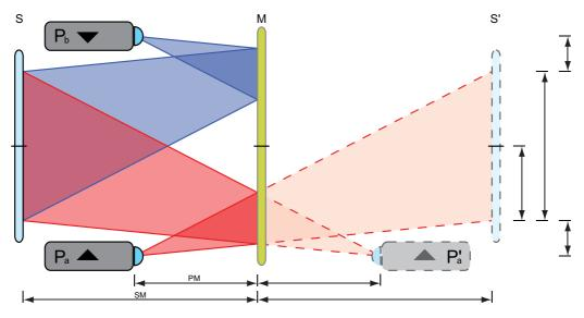
**Figure 4:** Layout of optical components to obtain an optimal, factory tuned rectangular image with two projectors. We take advantage of horizontal symmetry of off-the-shelf projector optics, and therefore can flip the second projector. The angle between projector and screen needs to be 90 degrees, and mirror needs to be parallel to the screen
