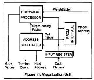
The address sequencer is a collection of incrementers, one for each the x-, y- and z-component of the raypoints, the depth-cueing factor and the raypoint number. Increments are added according to the skip distance. An inexpensive implementation uses an 8-entry on-chip SRAM, which holds the pre-computed increments, and which is addressed by the skip distance as shown in Figure 12.
