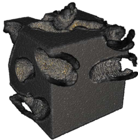
Figure 1: Volume representing a block of clay which has been plastically deformed.
