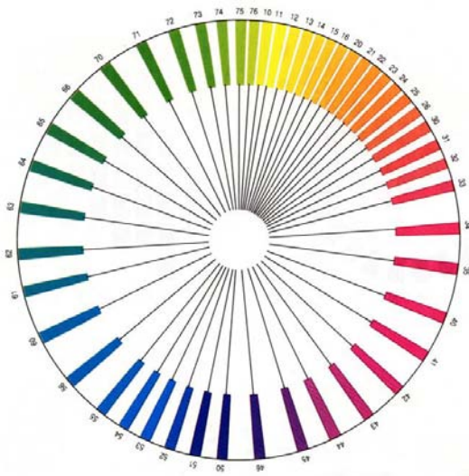
Figure 2: The aesthetically uniform 48 limit-colors of the Coloroid system built 7 hue groups with the non-uniform numbering: 10,...16, 20,...26, 30,...35, 40,...46, 50,...56, 60,...66, 70,...76, according the yellow, orange, red, purple, blue, cold-green, warm-green intervals
