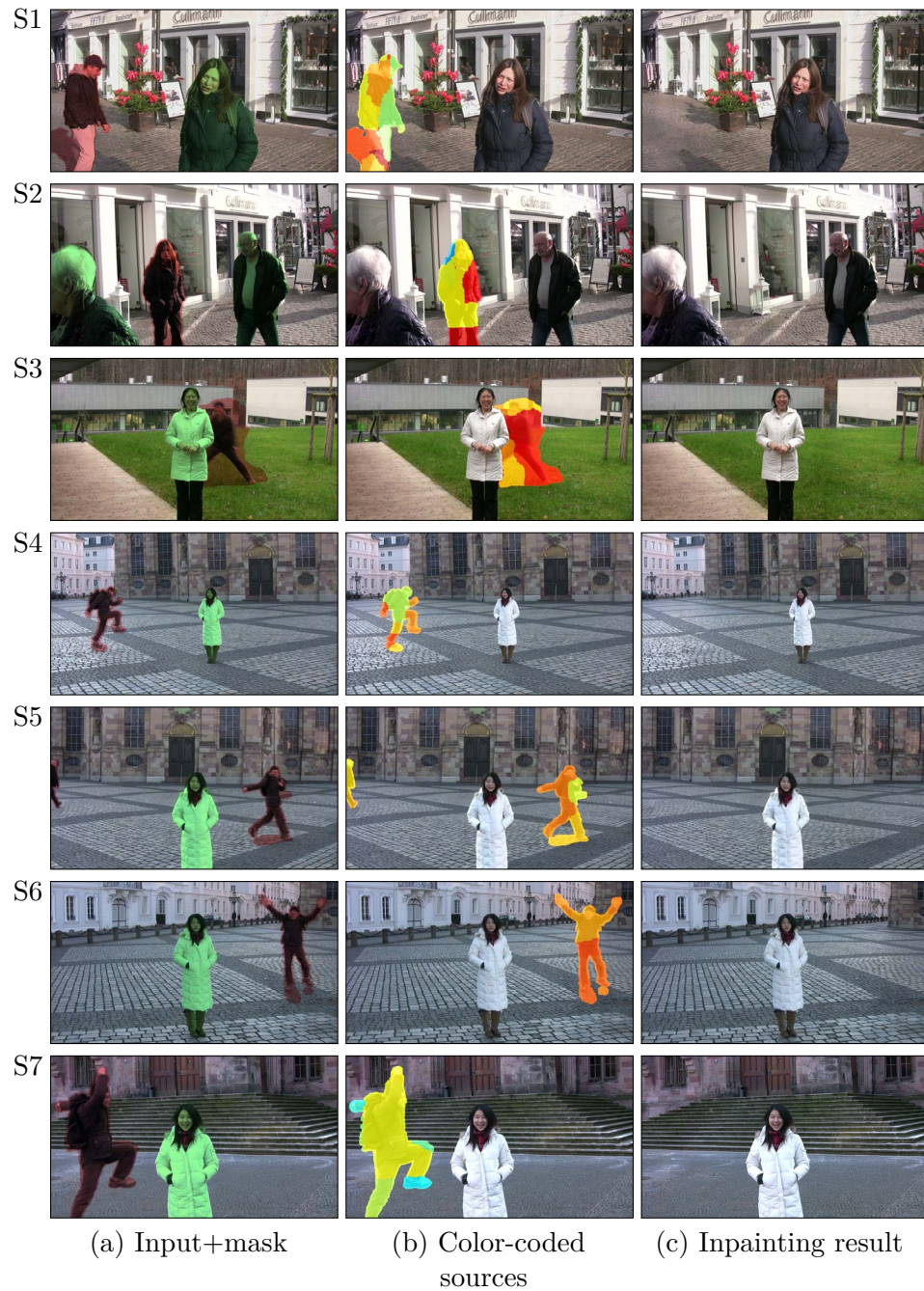
Figure 6.8: Inpainting results in the seven test sequences: (a) An input frame and the mask for the hole and dynamic objects (shaded in red and green, respectively); (b) visualization of the source frames obtained by minimizing Eq. 6.8, where each source is shown in a different color; (c) final inpainting result after compositing and gradient-domain fusion.
