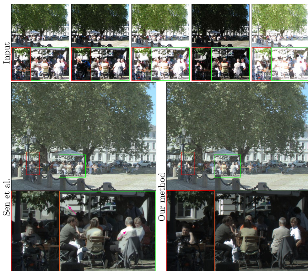
Figure 3.20: Comparison to Sen et al. on the Café terrace sequence (top). The first image was selected as reference by the method of Sen et al. Here, their method encounters difficulties extending the dynamic range of ill-exposed regions, which results in a washed-out appearance (bottom-left, indicated by arrows). In contrast, our method automatically selects well-exposed sources for every region.
