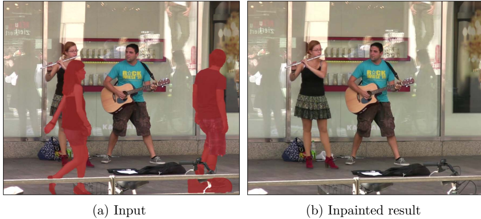
Figure 5.5: Inpainting of the duo sequence: (a) Overlay between one of the input frames and the mask of the object to be removed; (b) inpainting result using the proposed method.
