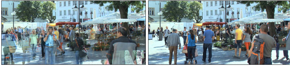
Figure 3.18: De-ghosting of the busy square using only the first three images shown in Fig. 3.10–top: (left) standard HDR reconstruction; (right) de-ghosting result. The legs of the rightmost person are not selected by the algorithm as the pants are under-exposed, and the background behind them is over-exposed. This type of semantic mistakes can be corrected interactively by the user (Fig. 3.19).
