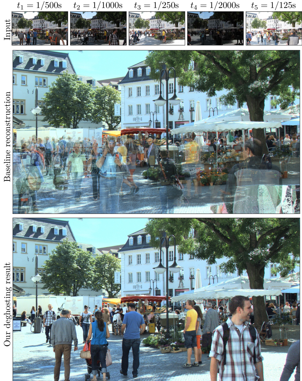
Figure 3.10: De-ghosting of the busy square sequence: (top) Five input images with different exposure time; (middle) standard HDR reconstruction where inconsistent pixels are included in the average; (c) de-ghosted HDR image using the proposed method. The labeling is corresponding to this result is shown in 3.11.
