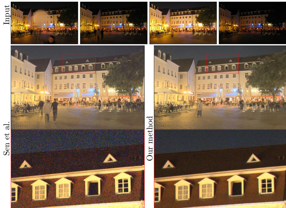
Figure 3.21: Comparison with the method of Sen et al. on the Square at night sequence (top). The second exposure was selected as reference for Sen et al.'s method. Due to noise, their method finds few similar patches in other exposures. This implies that the dynamic range cannot be effectively extended using other input images (bottom-left). Our method selects consistent sources with as low variance as possible, preventing the appearance of noise in the result (bottom-right).
