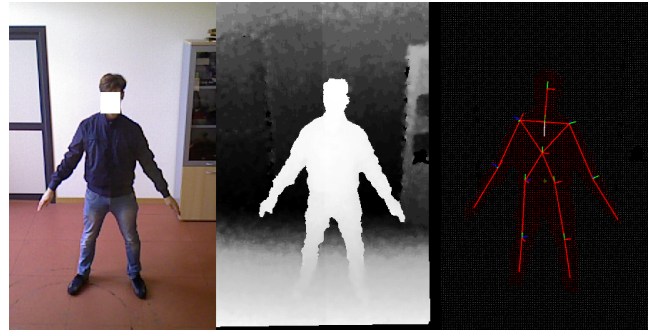
Figure 2: Example of RGB image (left) depth map (center) and skeleton (right) obtained by the sensor.
