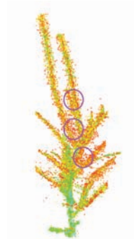
Figure 1: Point cloud from the inner crown of a leafless orchard tree. The point cloud is colored by intensity. The three marked areas show examples of noise where the separation of branches is even hard by visual inspection
