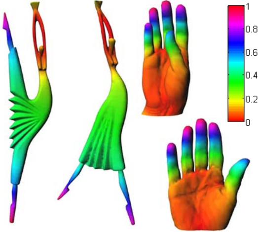
Figure 1: Color-coding of the conformal factor of two hand models and two dancer models from the AIM@SHAPE shape repository [ http://shapes.aim-at-shape.net/index.php ] (normalized to the range [0,1]).
