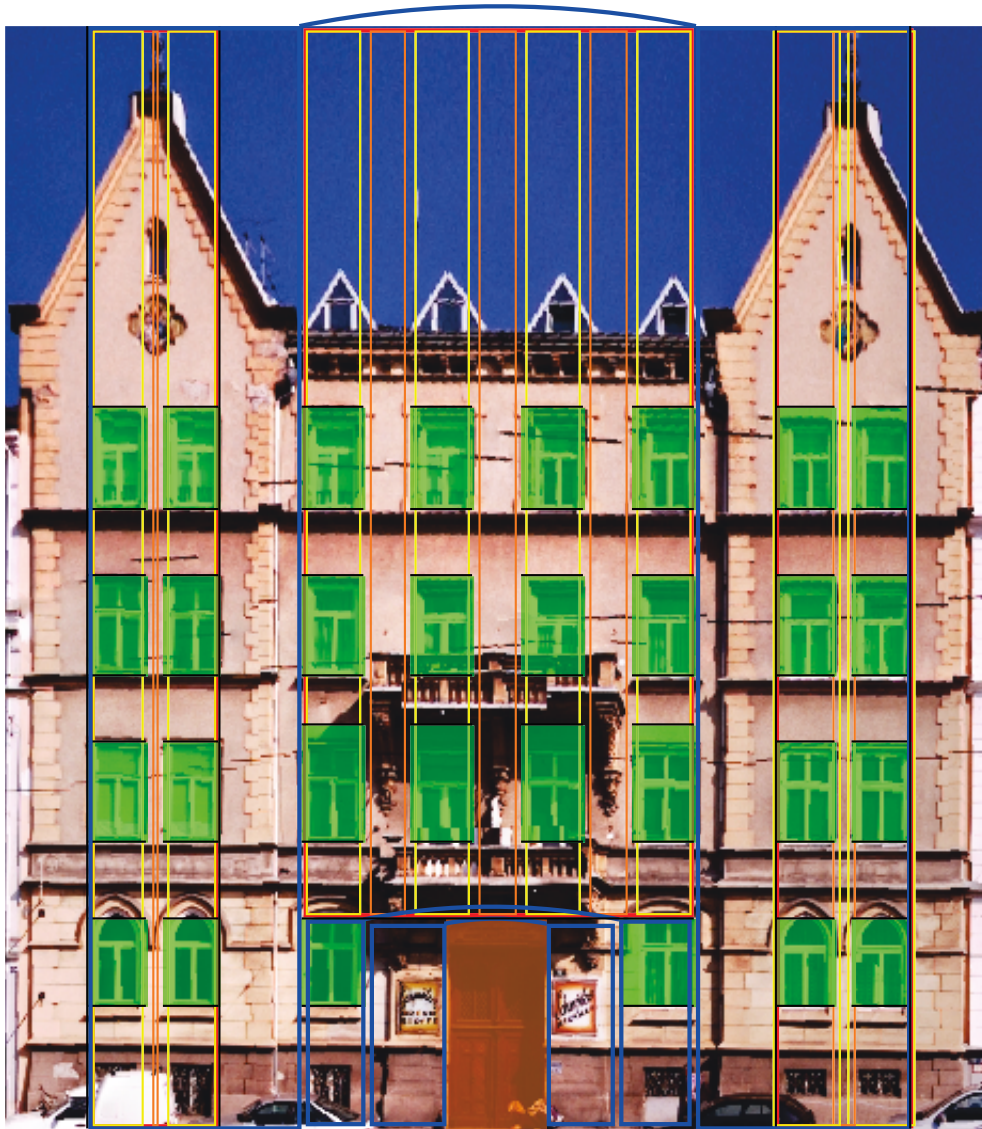
Figure 4.5: Parsed structure of a façade. Detected alternating repetitions of columns are shown as alternating rectangles of orange and yellow, symmetric side columns between a middle column are shown as blue rectangles (symmetric side columns) that are connected by a blue arc line. The result shows nested detected symmetries, such as repetitions inside a symmetric side column (left and right part). Also, the door has been parsed as a middle part that is surrounded by symmetric side columns.
