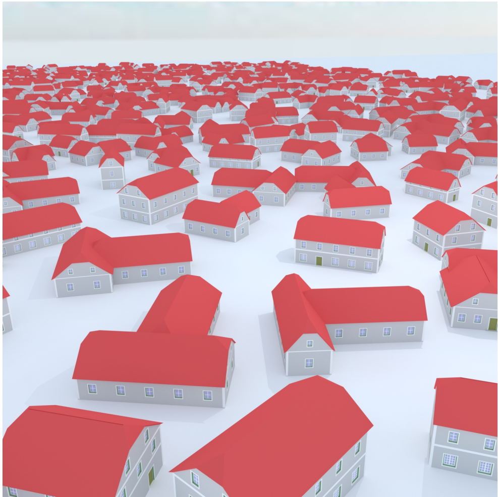
Figure 3.29: Variations of similar buildings can be generated using random intervals for values like width and height of a building. This randomly populated set of houses contains no two exactly similar houses - and is generated from two basic building layouts.
