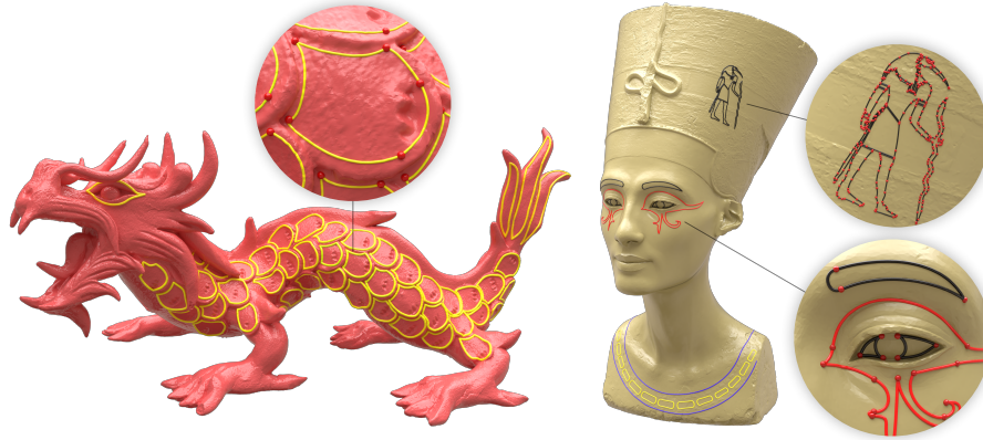
Figure 7.1: We propose algorithms to interactively edit Bézier splines on large meshes, including curve editing, curve transformations and import and editing complex SVG drawings. All computations occur in the intrinsic geodesic metric of the surface. All splines in this figure have been drawn interactively. Control points and tangents of curves under editing are shown in the zoomed insets. Asian Dragon \sim 7.2\text{M} triangles; Nefertiti \sim 500\text{K} triangles.
