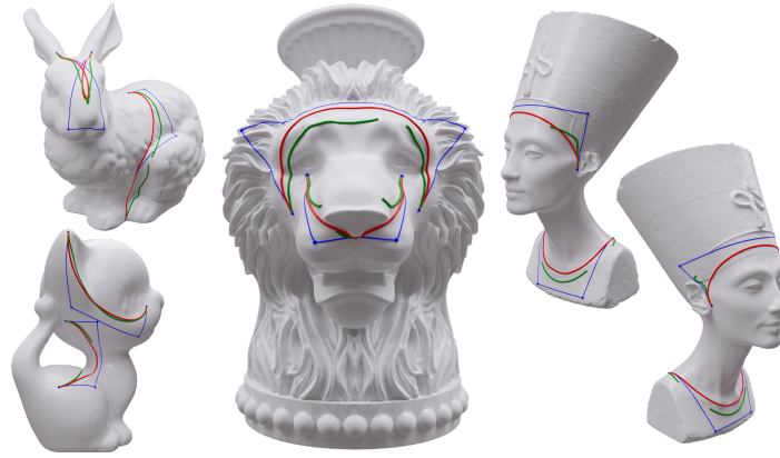
Figure 7.17: Comparisons between the WA method [PBDSH13] (green curves) on surfaces (bunny, kitten, lion, nefertiti) and our method (red curves). Control polygons are shown in blue. The WA curves may contain heavy artifacts (bunny), lose tangency at the endpoints (bunny, nefertiti), or be broken (kitten, lion, nefertiti).
