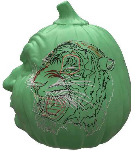
Figure 7.10: Example of importing a large SVG, made of 2056 curves, onto the pumpkin model, consisting of 394k triangles. Our algorithm takes 289 milliseconds to trace all curves.
