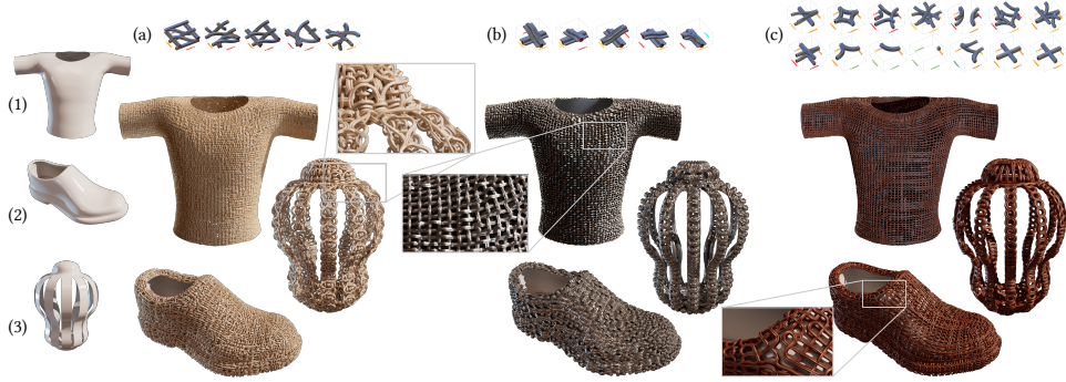
Figure IV.10: Once designed, the same tile set can be applied to various macro-surfaces.
